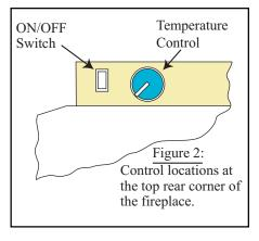
The Heater Control acts to turn the heater on and off as well as setting the comfort level in the room. Turning the knob clockwise from the off position will place the heater into operation. The further the knob is rotated clockwise, the higher the set point temperature. Turning the knob counterclockwise will lower the set point temperature. Turning it all the way counterclockwise will turn the heater function off.
